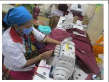
NC: Machine safety guard displaced
